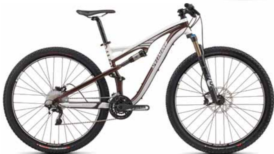
Camber Pro 29er: A pure 100mm XC Trail machine outfitted with FOX suspension and a custom SRAM double crankset.
